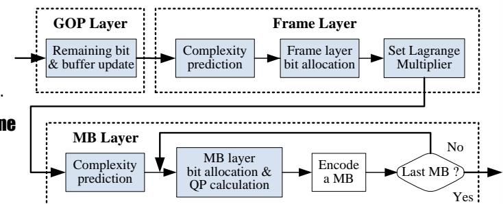
◆ Block diagram of encoding one frame with rate control
